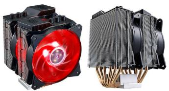
The MasterAir MA621P TR4 Edition is based around a dual-tower heatsink featuring aluminium fins. It is mounted on 7 heat pipes, with 6 in direct contact with IHS of the Threadripper processor. By default the cooler includes two 120mm MF120R RGB fans (each spinning at up to 1800 RPM), but customers can install one more fan to further improve performance. Cooler Master does not specify a TDP rating, but it should reach at least 250W if it is to cool big Threadripper CPUs.
