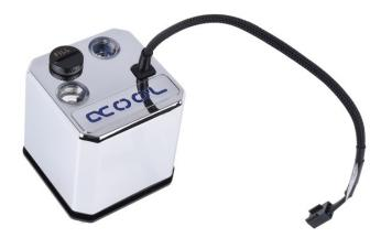
The Eisbaer Solo uses the DC-LT Low Noise Ceramic Pump found in many Alphacool products, with 4W power consumption and performance reaching 2600rpm. It has a 0.85m delivery head with a 70L/h maximum flow rate, while the reservoir features standard G1/4" threads for compatibility with "all standard water cooling connections. The reservoir is filled via the fill port on top of the housing, enabling quick cooling management.
