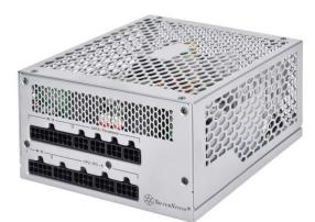
The NightJar NJ600 is ATX12V V2.4-compliant and rated at 600W output. The 80 Plus Titanium rating means it is at least 94% efficient under a 20%, 50% and 100% load, as well as at least 90% efficient under a 10% load. It features a modular design, with two EPS12V connectors allowing compatibility with high-end desktop motherboards (AMD Threadripper, Intel Core X) and 2P server/workstation platforms.
