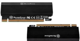
The EMC23 allows M.2 storage to run via PCIe connection, meaning users do not need to buy a new motherboard in case their PC lacks M.2 slots. It is compatible with AHCI over PCIe and NVMe (but not M.2 SATA connections) and houses a single PCIe M.2- 2230, 2242, 2260, or 2280 drive. Since heat is a concern with M.2 SSDs, the EMC32 includes x2 heat spreaders, thermal pad and x2 LEDs to monitor the activity of an installed SSD.
