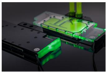
The EK-Vector RTX water block handles multiple Turing-based reference design graphics cards. It features a slim single slot design, and covers the entire length of the PCB. A "unique" cover over the block terminal reveals the graphics card model from the side. The cooling block comes in 8 versions, all featuring proprietary Open Slit-Flow micro-channels guiding cooling liquid to the GPU, VRAM and VRM (voltage regulating module), even with weaker water pumps.
