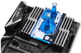
The cooling solutions claim to cover most of the Ryzen Threadripper surface for better thermal transfer, while cooling the power delivery with liquid flowing directly over the necessary components. Both monoblocks have a nickel-plated electrolytic copper base with an acrylic glass top, and come fully assembled with nickel-plated mounting screws and brass screw-in standoffs preinstalled.
