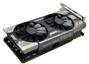
To cover the "cool" and "silent running" parts of the above claims the card features a 2.5 slot design with a larger, thicker heatsink compared to other EVGA offerings, including those with ACX 3.0 cooling and FTW enhancements. Such size minimises active cooling, keeping things relatively silent. It also features 10+2 power phases, 8+8-pin connectors, 235W power ceiling and two BIOS chips for simpler overclocking.
