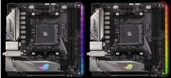
While built around the diminutive mini-ITX format, the two motherboards offer liquid-ready cooling, M.2 SSD heatsink, amped-up audio and addressable RGB lighting. They use the same 6-phase VRM design as full-size Asus ATX boards for AM4, and handle the higher memory clocks required by the platform through shorter traces in the dual-DIMM configuration.
