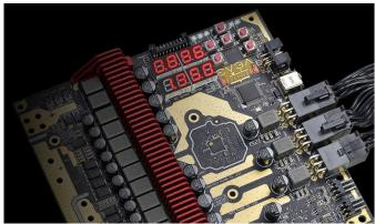
The Epower V provides customers with two fully-independent voltage outputs, with EVBot MKII facilitating on-the-fly voltage control. The board has an onboard VCORE and VMEM LED display, allowing one to quickly check status, while integrated EVBOT MKII buttons provide means to easily adjust voltages, upgrade the firmware and connect the EVBot to control the graphics card remotely.
