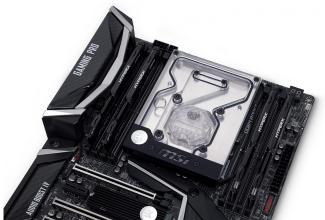
The cooling solution is compatible with the three Intel X299-based motherboards supporting the X-Series LGA-2066 processors, namely the MSI X299 Gaming Pro Carbon AC, Gaming Pro Carbon and Gaming M7 ACK. The monoblock uses an EK-Supremacy EVO engine to directly cool the CPU and MOSFET module, with liquid flowing directly over all critical areas.
