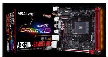
The board is designed to support the AMD Wraith Max CPU cooler, a high-performance cooling solution for the latest AMD CPUs, including Ryzen 7 processors. The Wraith Max has larger dimensions and weight, and to support it the AB3650N-Gaming Wifi motherboard features larger zones between the CPU socket and DIMM slots. As a result, it also allows users to install memory modules with larger coolers without any interference.
