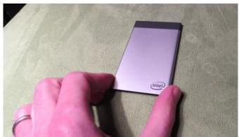
The Compute Card concept remains unchanged from that seen back in January 2017. A compact package fits an Intel system-on-chip, memory, storage and wifi/Bluetooth connectivity. One can slot the Compute Card in a variety of products, with examples seen at the show including a desktop PC replacement docks, laptops, smart TVs, VR headsets and even refrigerators.
