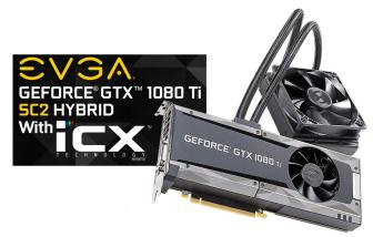
The liquid cooling takes care of the GPU, while the heatsink and fan keep the memory and VRM cool. The two cooling systems are combined with an array of thermal sensors and MCUs (iCX), and the company claims the result "gives you unbelievable GPU temperatures, sometimes cutting your GPU load temperatures in half."
