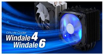
The naming is based on the amount of heat pipes equipped, thus the 4 and 6. Being the larger and more powerful model, the Windale 6 also gets the addition of a black radiator finish and blue LED illuminated fan. FSP says both coolers have direct contact 6mm diameter copper heat pipes for better cooling performance, as well as a patented solder-less louver fin assembly to further increase heat pipe effectiveness.
