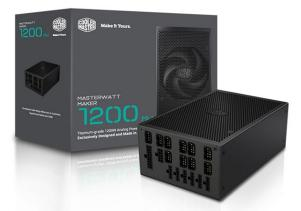
First revealed back at CES 2017, the MasterWatt Maker 1200 is made in Japan using a combination of Japanese and German components. It claims over 80 Plus Titanium efficiency and features a 135mm Silencio FP fan that only starts spinning once the supply hits 50% load.
