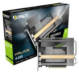
According to the company, the KalmX allows customers to play modern games at "full 1080p HD @ 60fps" while enjoying a "silent 0dB gaming environment." The card does this through a unique cooler, with chunky conducting metal construction connected directly to the CPU via copper base. Twin nickel-plated heat pipes pierce the copper block, bend round and thread through many nickel-plated fins.
