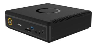
The Zotac Zbox line of miniature desktop PCs gets an upgrade to Intel Kaby Lake processors-bringing about the Magnus EN1070K, a machine capable of powering a VR headset despite being a little bigger than a Mac Mini.
