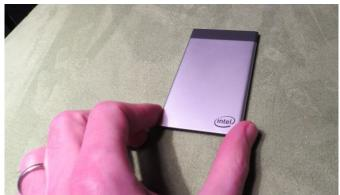
The compact Compute Card frame fits an Intel system-on-chip, memory, storage and wifi/Bluetooth connectivity. Chipzilla does not reveal the actual specifications as yet, but it promises a modular design customers will be able to configure with a range of processors, including 7th gen Intel Core CPUs with vPro.
