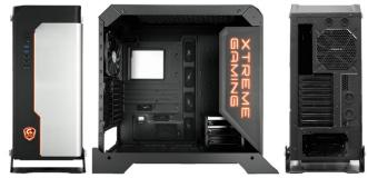
The XC700W measures 593.5 x 240.5 x 546.6mm and weighs 15.4kg before the addition of any components. Described by the company as a "perfect solution for a liquid cooling build," it has room for radiators up to 360mm in size or up to x3 120mm (or x2 140mm) fans if the user goes for air cooling. The chassis includes a 140mm rear fan fitted.
