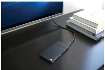
The Kangaroo carries a 2.24GHz Intel Cherrytrail (Atom Z8500) SoC, 2GB RAM, 32GB storage (expandable to 128GB via microSD card slot) and an onboard battery, making it able to handle light PC-style use and media playback. It measures 124 x 80.5 x 12.9mm, weighs 200g and connects to displays via HDMI, while Bluetooth 4.0 handles the addition of peripherals. Wifi takes care of the internet.
