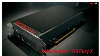
Based on the "Fiji" chip, the R9 Fury X has "the highest GPU memory bandwidth ever" through the use of <u>high bandwidth memory</u> (HBM), a GDDR5 RAM replacement consisting of vertical memory stacks. This allows for more memory within less board real estate, as well as for smaller graphics cards.
