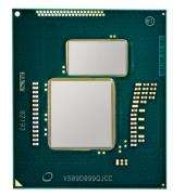
The processors also feature boosted integrated graphics via Iris Pro Graphics 6200-- the most powerful client processor graphics and media engine from the company yet. It features a 65W thermal design point (TDP) making it ideal for a broad range of PC form factors, including mini PCs and desktop All-in-Ones (AlOs).
