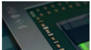
According to the company, GDDR5 RAM is not becoming any smaller-- on the contrary, it requires "significant board real estate," as well as greater amounts of power in order to meet the demands of increasingly faster GPUs. Enter HBM, a means to stack memory cells vertically instead of next to each other.
