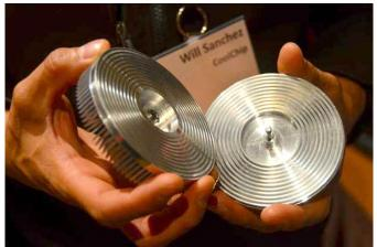
Kinetic cooling involves what essentially amounts to a rotating heatsink. According to CoolChip the rotation sucks air into middle before quickly expelling it in all directions through the fins, with a thin (a few microns) cushion of air separating the rotating heatsink from the base plate connected to the CPU.
