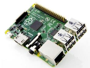
The first Raspberry Pi features a 26-pin GPIO. The first 26 pins on the Model B+ are identical to the original, allowing for backwards compatibility.
