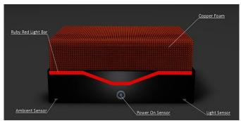
According to the company the copper foam offers a 500-fold increase in surface area over traditional heatsinks, and combined with air microcirculation it provides passive cooling efficient enough to keep outside surface temperatures below 50 degrees Celsius.
