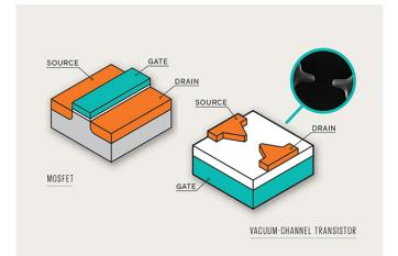
The vacuum-channel transistor is, essentially, a nano-scale vacuum tube. Like conventional MOSFETs it has a source and a drain, yet instead of a gate electrode it has... nothing. Electrons from the source to the drain when current is applied to the gate via "field emission," a process allowing for faster movements of electrons.
