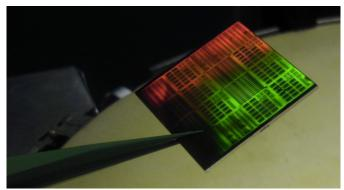
As described in Nature the circuit features acts as a radio frequency receiver, meaning it translates radio waves into information one can understand, as well as send signals back and forth. Tests involved sending a message on a 4.3GHz carrier signal saying "IBM," which was sent and received distortion-free.
