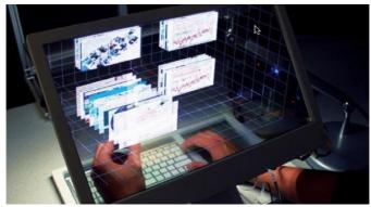
First developed at Microsoft Applied Science, the SpaceTop desktop unites 2D touch-based Uls, gesture-based control systems (such as Leap Motion or Kinect devices) and 3D visuals with the combination of transparent LED display, keyboard and a pair of cameras.
