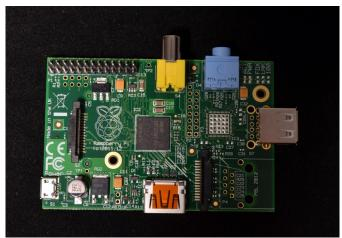
Just like its popular Model B brother, the Model A board carries a 700MHz ARM-based Broadcom CPU, but has just 1 USB port, 256GB of RAM and lacks an ethernet connector. It also cheaper (\$25, down from \$35) and uses even less power than the Model B.
