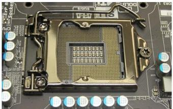
The current LGA socket is an 8-year old technology where the actual contacts are on the motherboard while the contact points are on the CPU.
