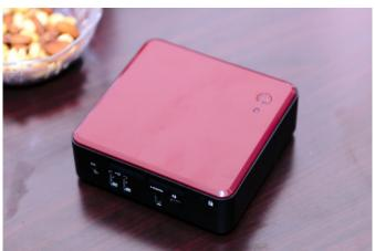
We all know compact PCs (such as the Via Pico ITX) are nothing new, but Intel pushes the smaller form factor futher. NUC carries a mobile Core i3 Ivy Bridge CPU, QS77 chipset (with integrated Intel HD 4000 graphics), x2 dual-channel DDR3 SoDIMM slots, mSATA and mini-PCle interfaces, all within a dimunitive motherboard and cooling assembly.
