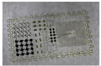
Current non-transparent semiconductors are based on silicon, gallium arsenide (GaAS) and other opaque materials. Metal oxide semiconductors, on the other hand, are not only transparent but also very efficient. However working on metal oxides demands very high temperatures (350C)-- too high for the plastic substrates flexible devices demand.
