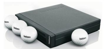
The M92p and M72e are a bit smaller than a Mac Mini, measuring 18 x 18 x 3.5cm. The diminutive cases (a bit thicker than a golf ball) fit x5 USB ports (with x3 USB 3.0 ports in the M92p) carry 3rd generation Intel Core processors and either HDD or SSD storage.
