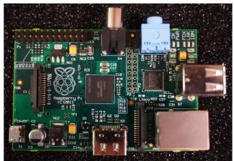
Designed as an affordable PC ideal to get children into computer programming, the Raspberry Pi is a tiny computer the size of a credit card. Currently a simple open board, it carries an ARM processor (running at 700MHz) on top of a Broadcom BCM2835 SoC, together with a Videocore 4 GPU the Foundation says is capable of HD playback.
