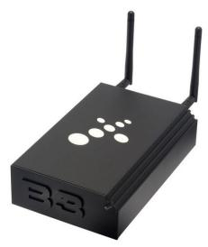
It carries a 1.2GHz ARM processor together with 512MB of RAM, while Excito says power consumption is as low as 5W. The device can handle up to 4TB of file sharing and storage.
