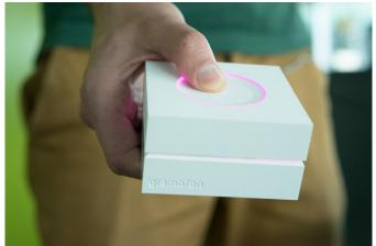
Essentially the Gramofon is a small router with built-in online music service support. It connects to audio systems via 3.5mm jack (it carries no speaker) and to home networks via either wifi or ethernet, and uses wifi to pair with mobile devices.
