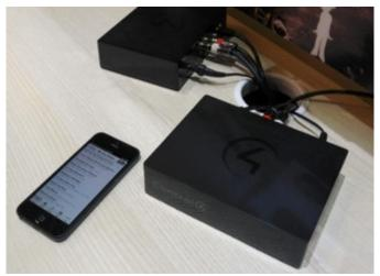
With Bluetooth, DLNA, Airplay, wifi and ethernet support, the Wireless Music Bridge streams audio from most, if not all, devices. It supports full metadata (including cover art) and allows access to connected content and devices through all Control4 interfaces, including TVs.
