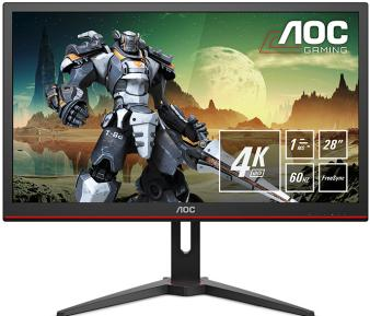
The display uses a "next-generation HDR-ready" TN panel with 300 nits maximum brightness, 1000:1 contrast ratio and 60Hz maximum refresh rate. As mentioned earlier the display supports FreeSync dynamic refresh rate technology, although AOC does not confirm whether it also supports Low Framerate Compensation.
