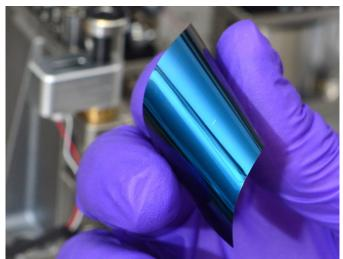
GST (aka Ge2Sb2Te5 or Germanium-Antimony-Tellurium) alloy is a phase change material (PCM), meaning it is able to change between two states with the application of heat, light or electricity. It finds use in rewritable CDs and DVDs, where laser pulses cause it to switch between amorphous and crystalline states.
