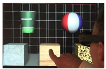
Called "Actuated 3D Display with Haptic Feedback," the monitor was shown off at Microsoft's TechFest 2013 event. It consists of an off-the-shelf multitouch 3D monitor mounted on a robot arm, both of which in turn are connected to the same PC.
