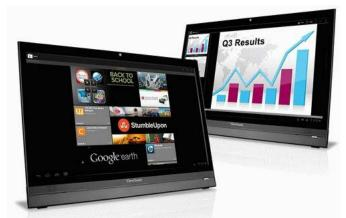
Making an Android LCD monitor involves little more than adding an ARM CPU and wifi radio to an LCD monitor. The hardware is futher bolstered with touch functionality, adjustable stand and the Android as OS, making what amounts to either a stripped-down AIO/oversized tablet capable of meeting customers' email/video/game needs.
