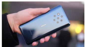
The 5 cameras share the same specifications, since each features a 12MP sensor and an f/1.8 lens. Two of the cameras shoot in colour, while the other three are in monochrome. To snap a photo, the cameras shoot at different exposures at the same time, before the phone merges all the image data into a single, ultra-detailed shot. Nokia even claims the individual cameras can shoot multiple exposures on their own, adding even more data to the final image.
