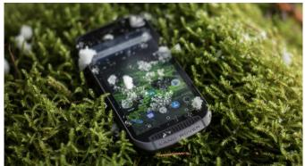
The work of British smartphone maker Bullitt (who made devices branded by the likes of Caterpillar, Kodak and JCB), the Explore includes a factory-fitted screen protector and protective casing allowing it to survive dives of up to 1.8m in salt water and drops of up to 1.8m. The phone also has an IP86 rating for splash, water and dust resistance, and includes the ViewRanger mapping app for customers wanting to take their Land Rover (the car, not the phone) off the beaten track.
