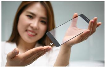
The fingerprint reader module fits in a space just 0.3mm deep. Being glass-covered it can be incorporated the underside of smartphone cover glass without need for dedicated buttons, pads or other exposed elements.
