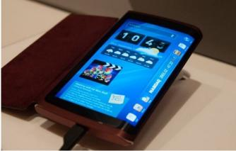
How can a display cover 3 sides? Through an evolution of Samsung's own curved-edge OLED displays, of course. The Galaxy Note Edge has such a display, if one wrapping around a single side of the device.
