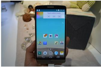
A device that's nearly all screen (thanks to impressively thin bezels), the G3 features a 5.5-inch 2560 x 1440 IPS display within brushed metal-effect plastic casing. The back is slightly curved, and the LG's unusual rear key returns in a smaller and flatter version sitting just beneath the camera.
