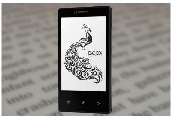
Seen at CeBIT 2014, the InkPhone carries a 4.3-inch elnk Flex display, 1GHz processor, 512MB RAM, 4GB storage and a 1800 mAh battery promising up to 2 weeks of use on a single charge. How so? Through the elnk display, of course.
