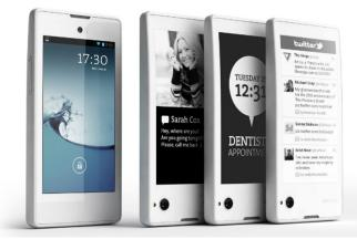
The device remains fairly unchanged from when we first saw it back at CES 2013. It still features a 4.3-inch 1280x720 LCD display on the front and a same-size 640x360 EPD on the back, providing what Yota calls an "always-on, low-power display."
