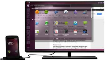
The idea is similar to the Motorola Atrix, which used the Motorla Webtop OS and the hardware Lapdock. However Canonical pushes the concept even further by having the phone switch to a different OS (ARM Linux) when docked via HDMI and USB ports.
